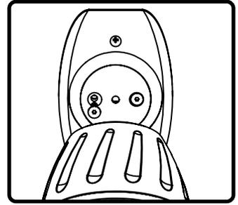
4. Attach speaker to mounting plate with supplied fasteners. No wiring is necessary because signal wire contact is made when speaker is screwed in place.
