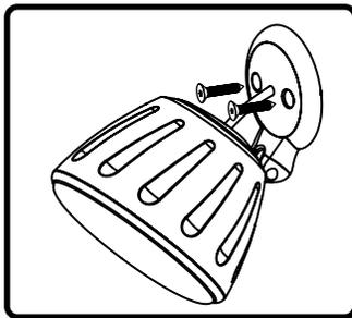
5. Attach speaker to surface using installer-supplied fasteners.
