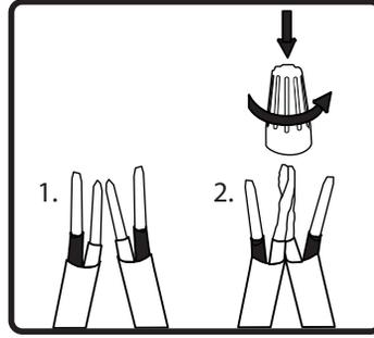
3. Connect the speaker wire to the input signal wire. Red is positive, black is negative.
