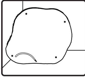
2. Locate speaker wire on the underside of the speaker. Strip wire ends if necessary.
